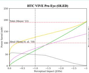
Considering eye tracker power, brightness rolloff saves less power than uniform/dichoptic dimming.
